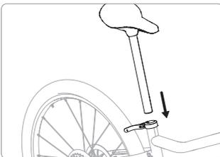
Insert the seatpost and position it at the correct height. Observe the positioning zone (A, B or C) and correspond the letter to the handlebars to ensure they are in the optimal position.
