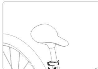
Close the quick-release lever completely.
